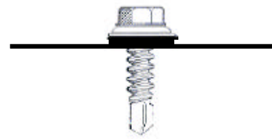
TOO LOOSE! SEALANT IS NOT COMPRESSED TO FORM SEAL
