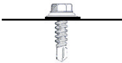
CORRECT DEGREE OF TIGHTNESS (NOTE SLIGHT CIRCLE OF SEALANT)
