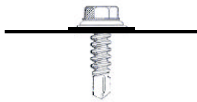
TOO TIGHT! SEALANT SQUEEZED TO THIN, EXTRUDES FAR BEYOND FASTENER HEAD
